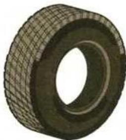
Patterns on the surfaces of tyres are made to increase friction between the tyres and the road surface.
