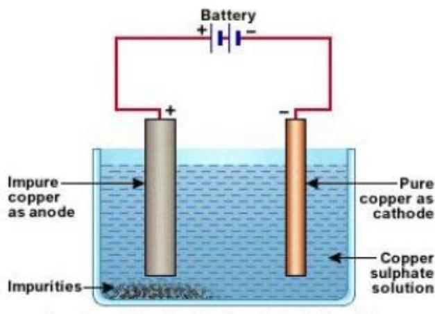
Fig.2. Electrolytic refining
